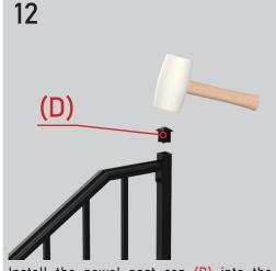
Install the newel post cap (D) into the upper post top by gently tapping it in with a rubber mallet.
