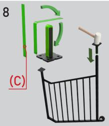
Remove the dry fitted Post Mount Bracket, and locate the green snug strips (C) included in the kit. Wrap the snug strips to engage the sides of the post. Ensure the snug strips are positioned side to side - NOT FRONT TO BACK. Using a mallet, tap the Post Mount Bracket and snug strip into the lower post.
