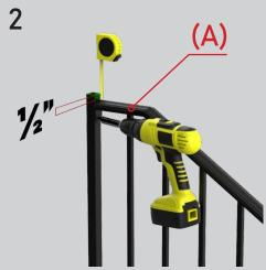
Place a mark on the newel post ½" down from the top of the post. Center the handrail mounting clips to the newel post and align the top of the handrail cap (A) to the ½" mark. Using the supplied ¾8" driver bit and your screw gun, with firm pressure, screw the self drilling screws through the handrail mounting clip into the newel post. The screws are self drilling and will cut into the newel post.
