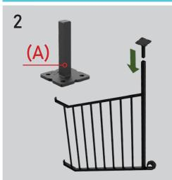
Insert the Post Mount Bracket (A) into the bottom of the lower post WITHOUT SNUG STRIPS. This will be temporary to get correct measurements. The snug strips will be used in a later step.
