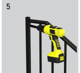
Once the rail is sitting plumb in all directions, use the supplied 3/8" driver bit and your screw gun, with firm pressure, to screw the self drilling screws through the handrail mounting clips into the newel post. The screws are self drilling and will cut into the newel post.
