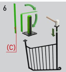
Remove the dry fitted Post Mount Bracket, and locate the green snug strips (C) included in the kit. Wrap the snug strips to engage the sides of the post. Ensure the snug strips are positioned side to side - NOT FRONT TO BACK. Using a mallet, tap the Post Mount Bracket and snug strip into the lower post.
