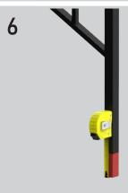
Remove the Post Mount Bracket from the bottom post, and measure from the bottom of the post. Take the measurement from step 5 and mark onto the bottom post. Make a cut at this mark. Touch up any exposed steel using the included touch up paint.
