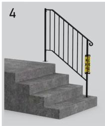
Take the rail assembly, and place it where it is to be mounted on the steps. Each post should be a minimum of 2" from each side of the step. Use a level to ensure plumb in all directions. This will cause a gap underneath the top post, which will be corrected.
