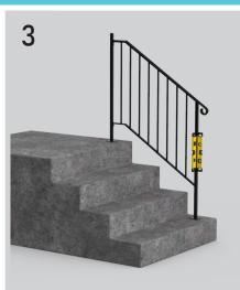
With the Post Mount Bracket inserted, dry fit the rail and top post on the steps. Place the posts at least 2" from each side of the steps. DO NOT ATTACH THE TOP POST AND RAIL YET. Use a level to ensure the posts are plumb in all directions.
