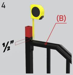
It may be necessary to cut the back post before connecting the rail. Mark the post  $\frac{1}{2}$ " up from the top of the handrail cap (B). Make a cut at this mark. The excess material can be cut any time prior to inserting the newel cap.
