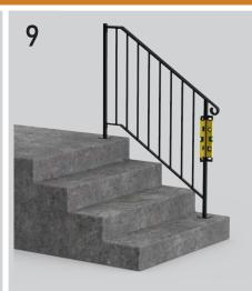
Place the handrail assembly on the steps in its final location. Verify plumb in all directions. It is advisable to step back and look at the handrail placement to ensure it is setting in an appropriate location. For masonry step applications, it is advisable to place the handrail a minimum of 2" from all edges.
