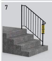
Replace the lower post mount bracket into the bottom of the post and verify your handrail sets plumb in all directions.
