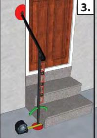
It is helpful to check and recheck for plumb both directions multiple times.
