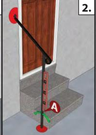
Place a level on the front surface of the post (A). It is not necessary to plumb the post side to side yet.
