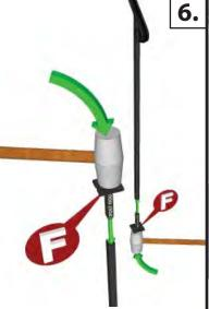
Slide the post mount and snug strip assembly (F) into the bottoms ( $\rightarrow$   $\rightarrow$ ) of the rail posts.
