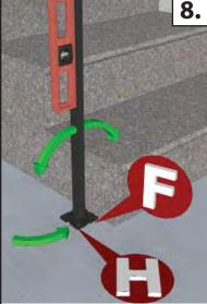
To help plumb the rail posts side to side  $(\leftrightarrow)$ , use the stainless steel washers **(H)** provided to shim underneath the mounting plates **(F)** before fully tightening the anchors to your steps.
