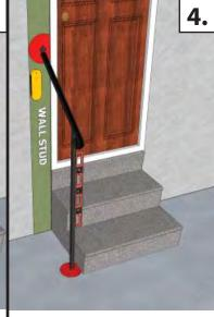
adequate support within the wall where the handrail is touching the wall.
