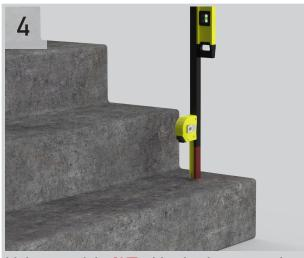
Set the rail back onto the steps and check that the rail post are sitting plumb.
